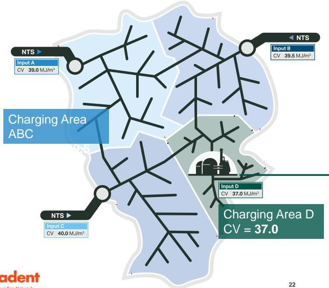
Measured CV assigned to Supply **Meter Points**
