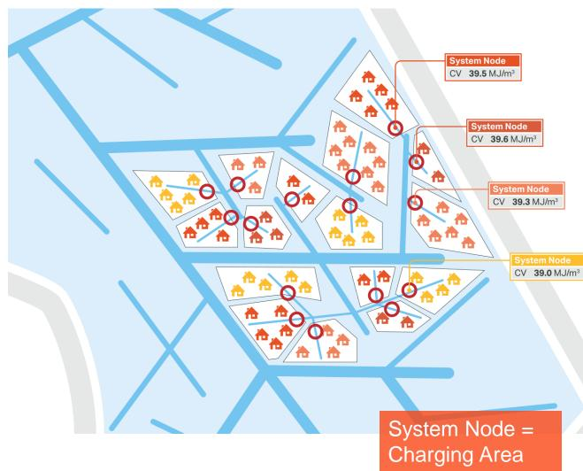
Measured CV and volumes at LDZ offtakes from NTS are inputs to online LTS model
